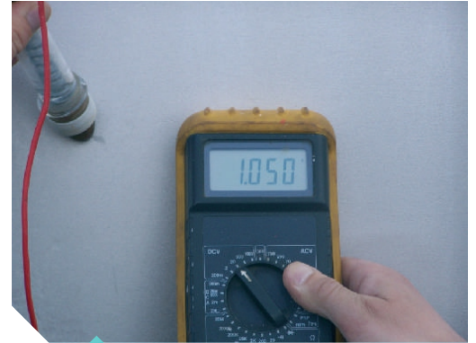
Control of the passive film quality with the potential meter
