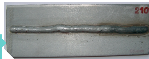
Sample of 2101 duplex steel with an overweld Test for heat tint and oxide scale removing
