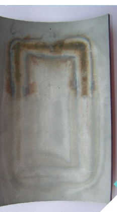
Sample of 2205 duplex steel with an overweld Test for heat tint and oxide scale removing
